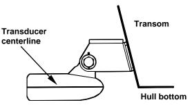
Align transducer centerline with hull bottom.
